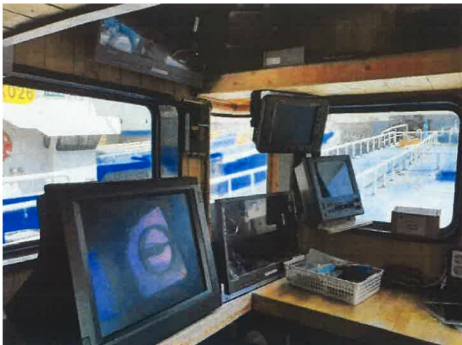
Radar,Fish Finder,GPS Plotter
